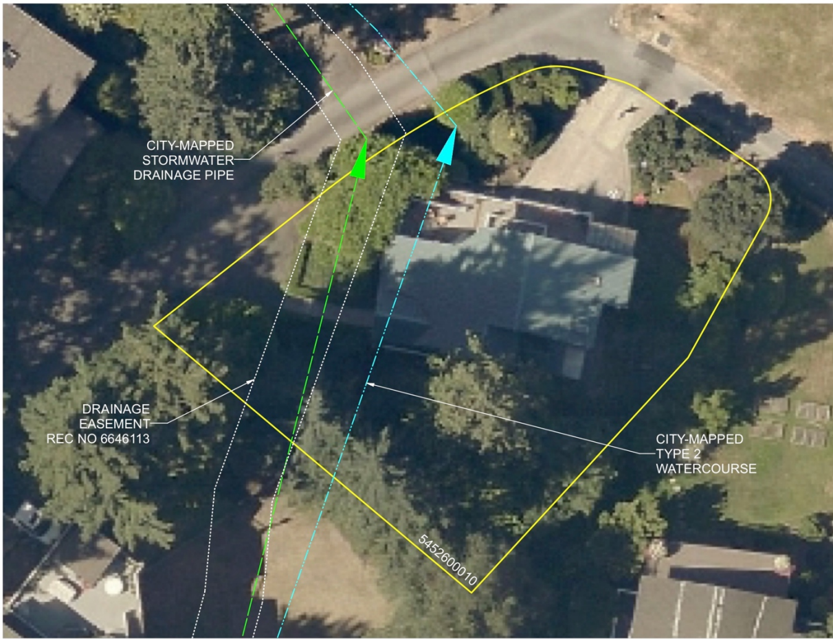
Figure 3 - Aerial photo of subject property with Mercer Island GIS Portal mapped Type 2 watercourse and stormwater drainage pipe, and recorded drainage easement.
